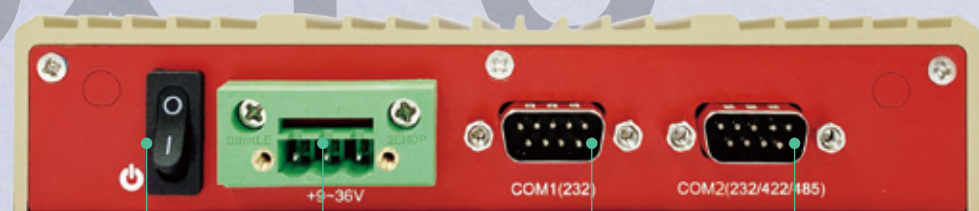
Power Button 3 pins terminal block power connector COM RS-232 COM RS-232/422/485
